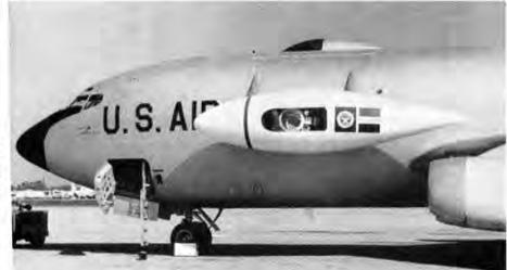
THE ALOTS POD fixed to the cargo door of the NKC-135. Large lens is the telescope, smaller ones to the right are the TV lenses.
